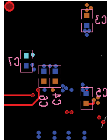
Figure 53. Bottom Layer Decoupling
